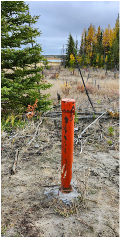
Photo 12: Shallow Well for Monitoring Groundwater
