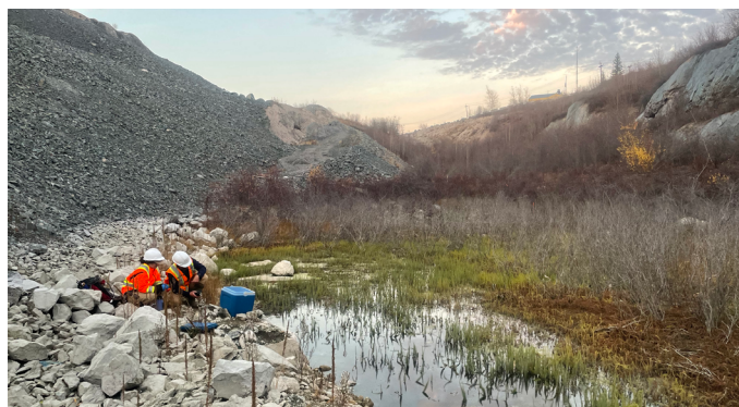
Photo 36: Study of Inflow from Baker Creek to C1 Pit, 2023 Upper photo: environmentally friendly dye used in Baker Creek in late Fall Lower photo: monitoring at base of C1 Pit to check if dye entered the pit
