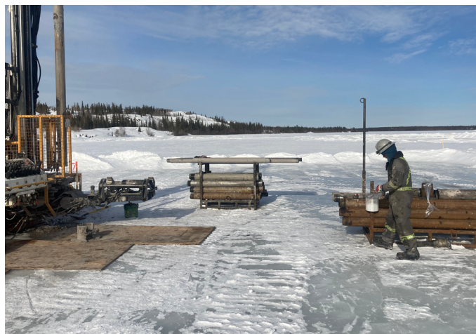
Photo 38: Geotechnical Investigation within Foreshore Tailings Area (drilling into the tailings underwater to check for tailings layer thickness and property using a sonic drill)
