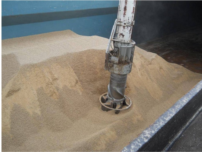
Fig 5 An example of small-scale sweep arms being used on a ship unloader with wood pellets.
