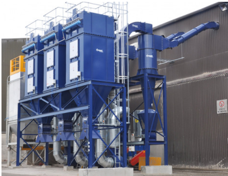
Fig 7 An example showing cyclones (right) feeding forward into baghouses (left) (c/o impactairsystems.com)
